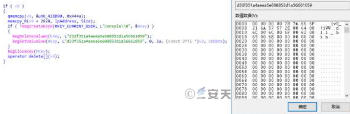
Figure 3-7 Write Shellcode contents to the registry 3-7
