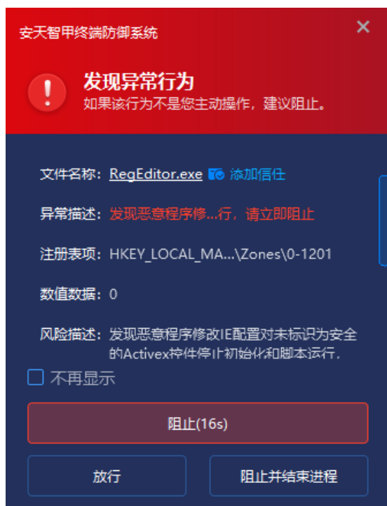
Figure 4-3 Intercepting and sending an alarm during an abnormal registry operation2
