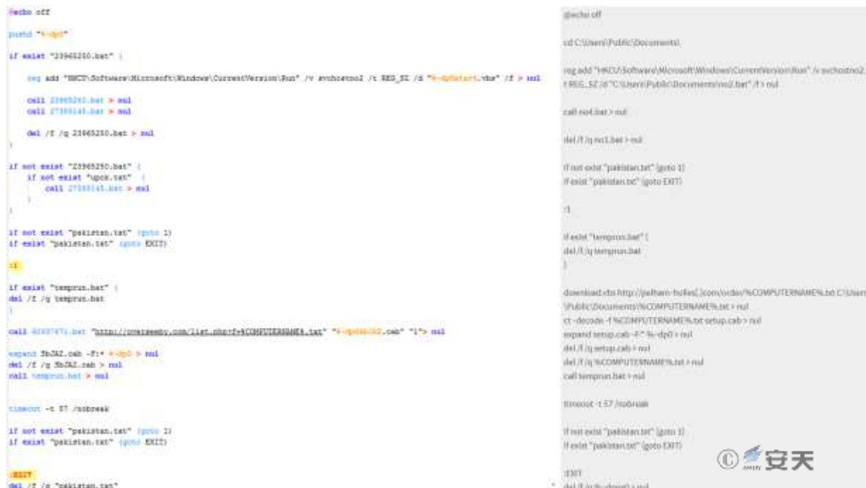
Figure 3-3 Scripts used for file calls and downloads in this attack campaign (left), scripts used for file calls and downloads in previous attack campaigns (right) [2]
