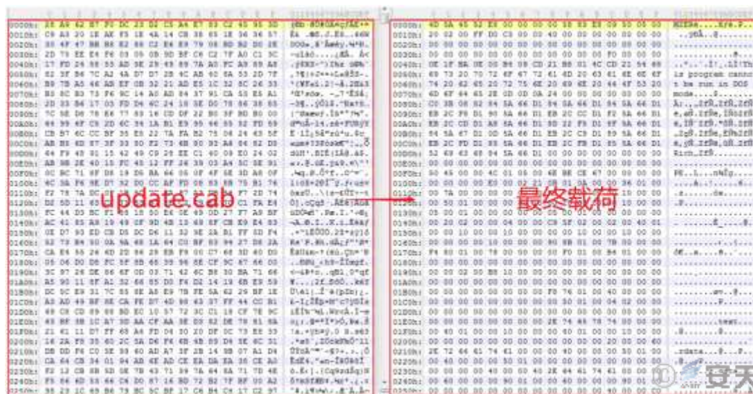
Figure 2-13RC4 decryption of the update.cab file to obtain the final payload
