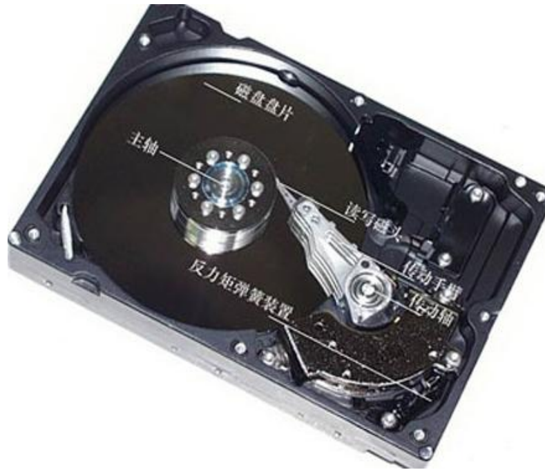
Figure 9 The composition and structure of the mechanical hard disk
